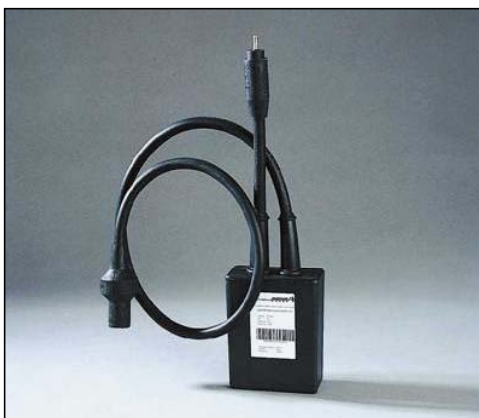
Fig. 2 Safegate Lamp Monitor and Switch (LMS) allows control and monitoring of every lamp on the airfield. The LMS simply plugs in between the isolation transformer and lamp.
