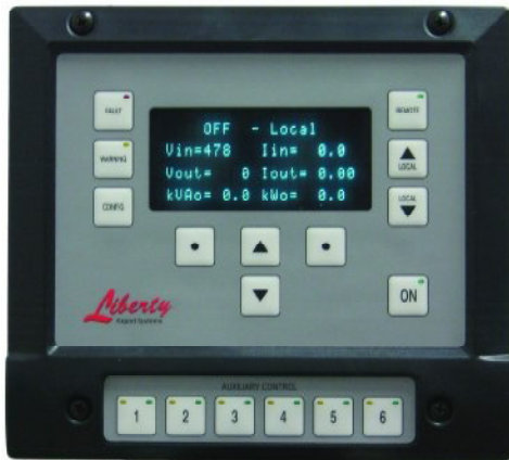
Fig. 2 Freedom Series regulator keypad with 6 auxiliary control switches and status lights for direct CSS control.
