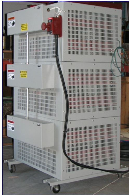
Fig. 1 30 KW, 20A Resistive Load Bank with castors.
